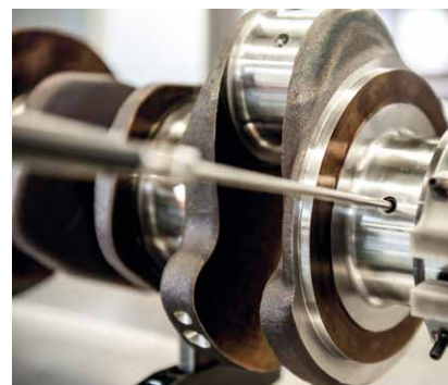
Piercing the oil duct
