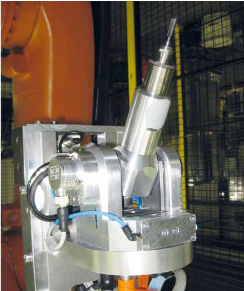
Sampas milling head with integrated measurement system
