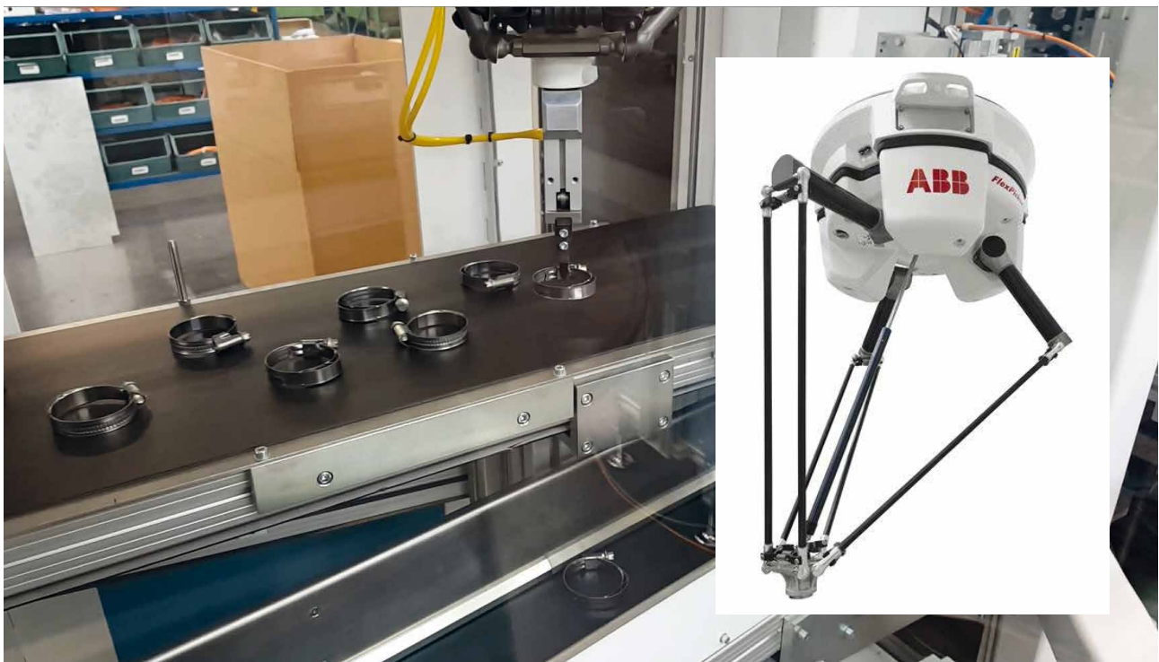
Robot picks up pipe clamps from the moving conveyor belt.
