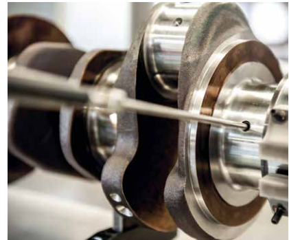
Piercing the oil duct
